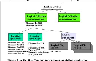
Figure 2: A Replica Catalog for a climate modeling application.
