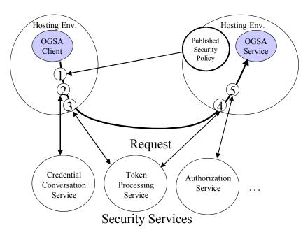
Figure 3. Example of a secured request in the OGSA security model. The steps are described in the text.
