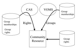
Figure 8: Difference between CAS and VOMS models. VOMS issues group memberships, which are mapped to rights by a resource. CAS issues rights directly.
