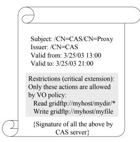
Figure 5: Example of a restricted proxy certificate, simplified for clarity, issued by initial CAS prototype. The certificate identifies the user as a member of the VO and the restrictions enumerate the user's rights within the VO.
